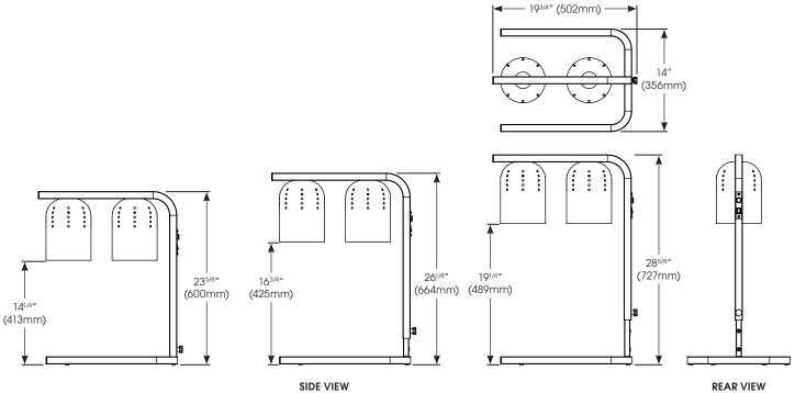
**OVERALL DIMENSIONS** SHIP MODEL DESCRIPTION VOLTS ΗZ WATTS AMPS PLUG WEIGHT LENGTH DEPTH HEIGHT 23-5/8" EHL-2C (600mm) (Silver) Electric 19-3/4" 14" 26-1/8" 6.61 lbs Freestanding 120 50/60 500 4.2 NEMA 5-15P (502mm) (356mm) (664mm) (3 kgs) Heat Lamp EHL-3C 28-5/8" (Black) (727mm)
