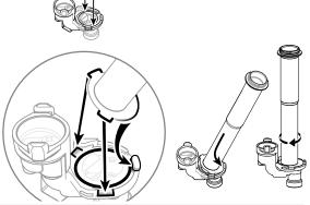
NSTALL MEDIUM O-RING onto discharge tube.
