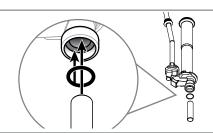
10 INSTALL LID by sliding smaller lid hole over discharge tube.
