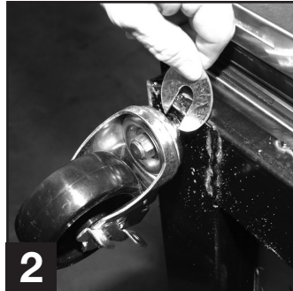
2 For leveling, insert the shim between the castor and frame rail.
