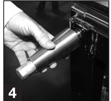
4 Thread leg into cabinet bottom frame rail.
