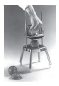
8. Push handle down with a quick firm stroke until the pusher head stops. The product will be completely diced. See figure 4.
