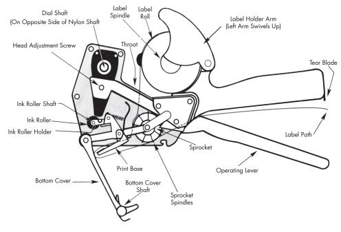
Facing side plate is shown removed for diagram purpose only.
