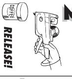
Fully release operating lever to obtain printed label at the dispensing head.
