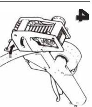
Insert labels into the channel on left side of labeler and close stamp receiver.
