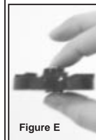
Bearing sleeve and impeller should spin freely when held like this. If parts do not spin freely or are worn, unit will not cool properly and worn parts may damage machine.
